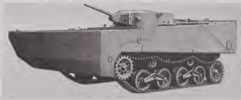
FIGURE 21. Japanese "ground-up" light tank design for intermittent amphibious operation. Bow and stern pontoons are closely integrated with main hull but are readily jettisoned for land operation. Twin screw propelled. Model shown captured summer 1944.
